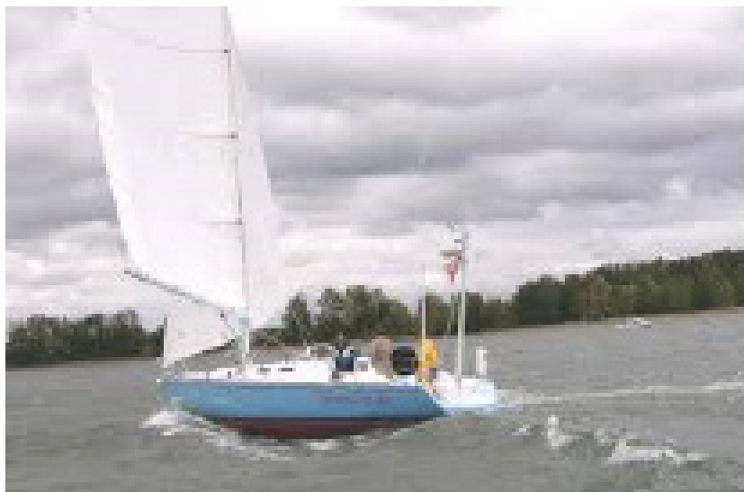
Boat At Hull Speed Notice the Bow and Stern Waves
